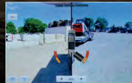
NEW TRAILER REVERSE GUIDANCE This available feature provides camera views and steering guidance graphics to assist in backing up and parking a trailer.
